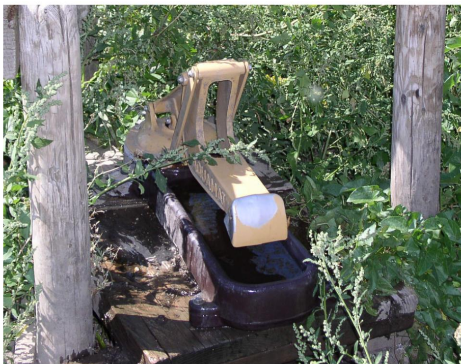
Animal-activated water pumping system
