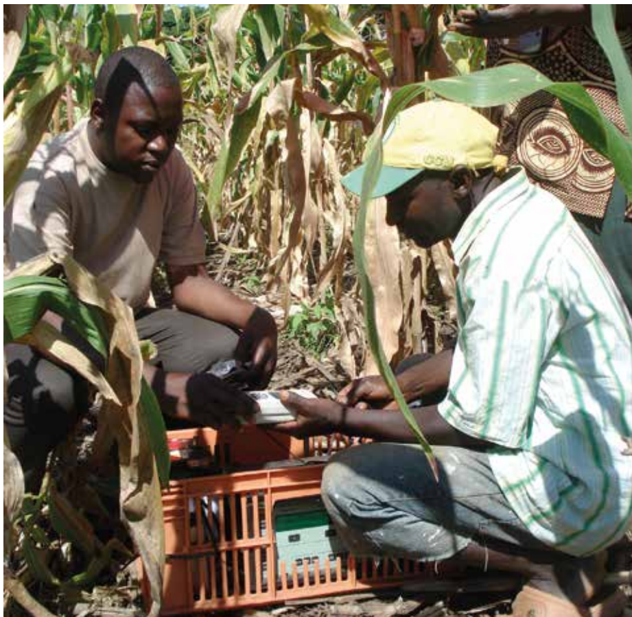
Figure 19. GHG emissions measurements with chamber techniques.
